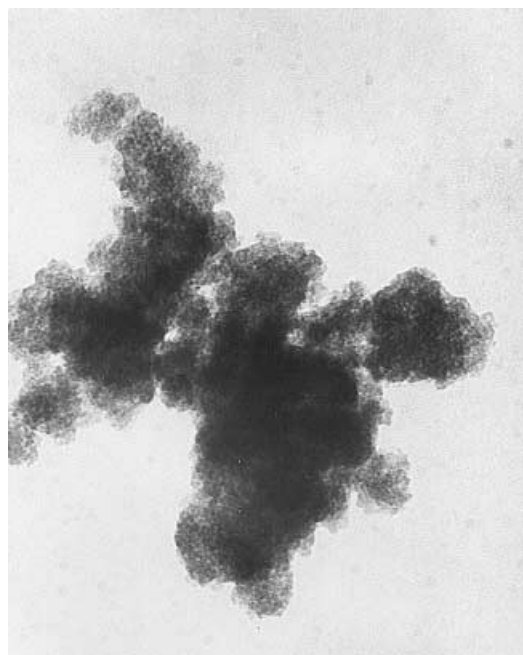
Figure 6. TEM micrograph of a \gamma -Fe 2 O 3 sample heat-treated at 250°C.
